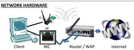
All clients need an NIC to connect to a ROUTER. This could be a wireless adapter or a network card. The Router in this simple connection can host multiple clients, but more advanced hardware is needed for bigger networks
